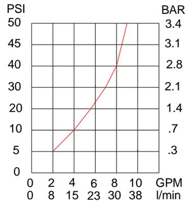
**CAUTION!** All thermostatic water mixing valves have limitations. They will NOT provide the desired accuracy outside of their flow capacity range. Consult the Flow Capacity Chart and DO NOT OVERSIZE. Minimum flow must be no less than as indicated.
