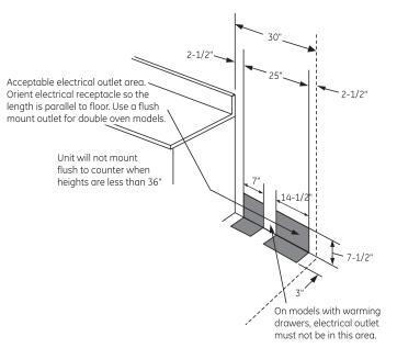
**NOTE:** Use a 4' power cord to prevent interference with unit when installing.
