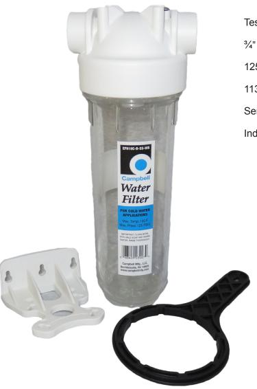
Tested to NSF standards as listed by IAPMO <sup>3</sup>/<sub>4</sub>" inlet/outlet, 316 stainless steel inserts 125 psi maximum operating pressure 113°F maximum operating temperature Service wrench and bracket included Individually boxed, master carton (12)
