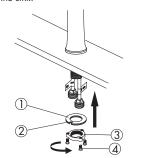
Install Rubber Washer (2) between Lower Drain Pipe (3) and Drain Body (1). Thread Lower Drain Pipe (3) onto Drain Body (1).
