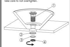
Slide Rubber Washer (1), and Metal Washer (2) onto threaded shank of faucet. Thread Mounting Nut (3) onto faucet shank until hand tight. Use phillips screwdriver to tighten Mounting Screws (4), securing the faucet to the sink.
