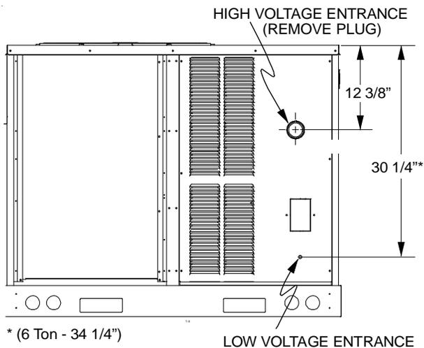
**NOTE:** Field-supplied conduit may need to be installed depending on unit/curb configuration. Use #18 AWG solid conductor wire whenever connecting thermostat wires to terminals on sub-base. DO NOT use larger than #18 AWG wire. A transition to #18 AWG wire may be required before entering thermostat sub-base.
