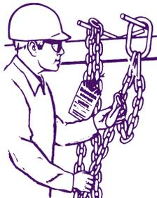
2. Know the load — determine the weight, center of gravity, angle of lift and select the proper size and type of sling.
