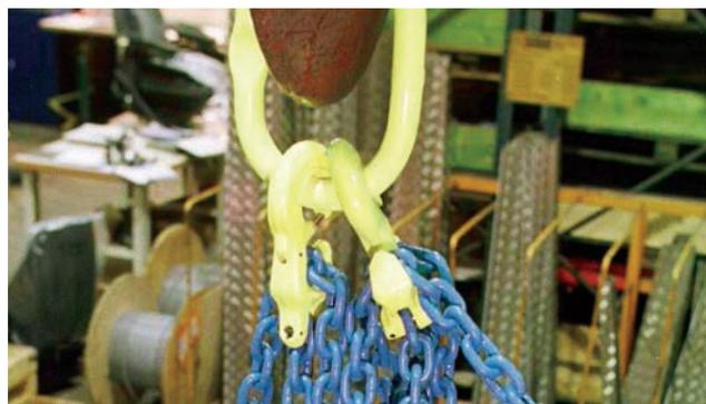
**Figure 3.** “A three-leg, fully adjustable sling.”
