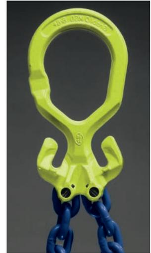
**Figure 1.** The GrabiQ Master Grab combines a master link, master link connectors for two legs of chain, and two shortening hooks into a single fitting. The shortening hook can also be used to create loop legs.
