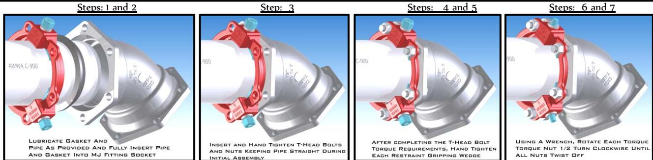
1. Insure the beveled pipe end to be joined and mechanical joint socket are clean and free of debris. Slide the Red TUF Grip onto the beveled end of the pipe to be restrained. The TUF Grip compression lip extension must be toward the beveled end of the pipe being restrained.
