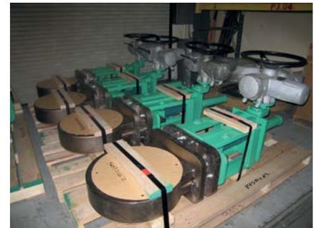
Coatings from Pentair are used on all our knife gate and slurry valve products. This example is a 900 PSI L&M valve M345 [HP] with SSEC coated body for use in a severe mining application.
