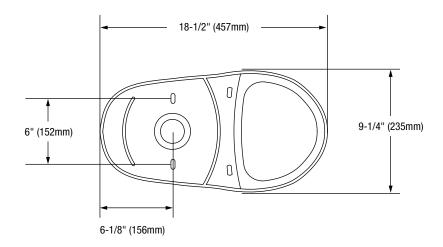
Note: All dimensions and specifications are nominal and may vary: Dimensions of 8" and greater have a tolerance of +3%. Dimensions less than 8" have a tolerance of +5%.
