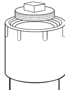
3. Hand tighten the Sewer Popper™ in place of the plug.
