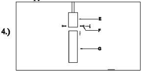
Step 4: Insert glass (G) into cup (E) and secure using two screws (F) provided.
