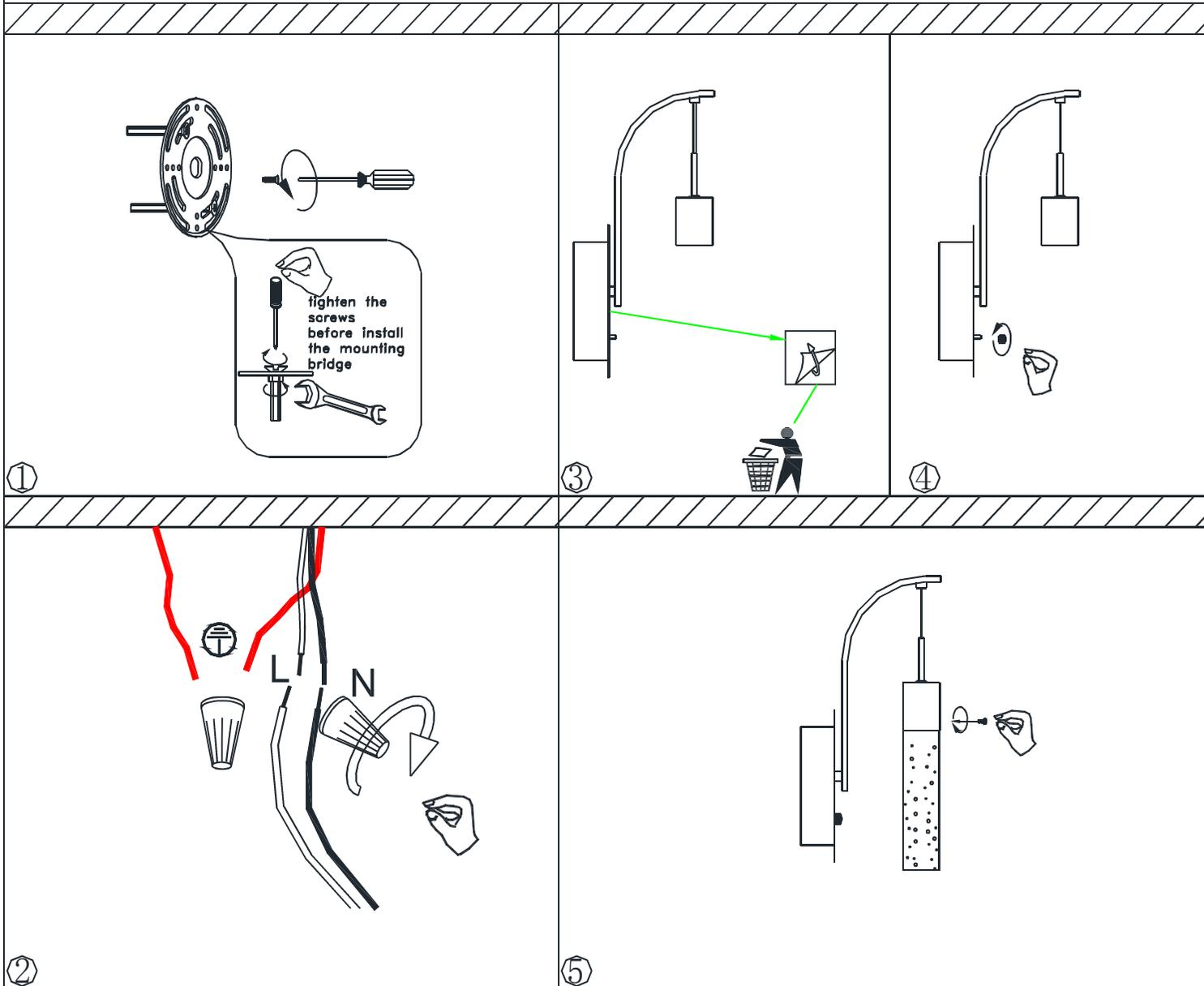
1. Turn breaker off for circuit on outlet where fixture is to be installed.
