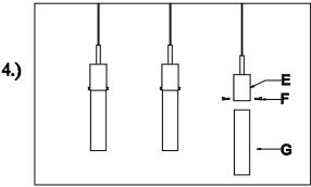
Step 4: Insert glass (G) into cup (E) and secure using two screws (F) provided.
