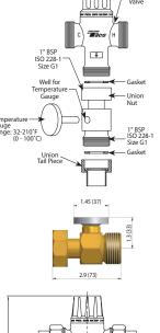
5000 Series Mixing Valve Dimensions Dimensions for reference only
