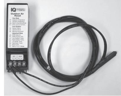
Intelligent Hydronic Control Operating Setpoint is normally set to the High Limit Setpoint. However, when an IQ Outdoor Reset Option Card is installed the Operating Setpoint may be reduced to the outdoor reset or Domestic Hot Water (DHW) Setpoint. When an IQ Outdoor Reset Option Card is added the following user defined setpoints are available:
