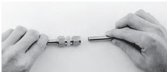
Simply insert the tubing into the assembly, making sure the tubing seats firmly against the shoulder of the body and the nut is finger tight. High pressure applications and high safety-factor systems. Further tighten the nut until the tube will not turn by hand or move axially in the fitting.
