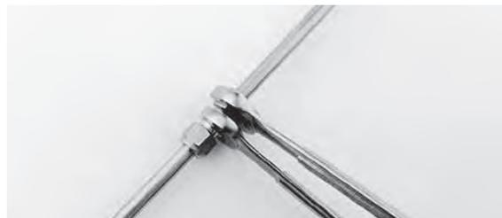
Tighten nut with wrench the additional number of turns indicated above, while holding the fitting body with a second wrench.
