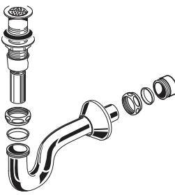
10. Connect the trap to the drain assembly, (not included) hand tighten and check for alignment. Trim the tailpiece and horizontal leg of the trap to fit your specific area. Secure joints for a watertight seal.
