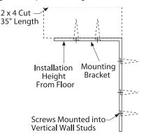
• Secure the bracket with wood block to the back wall so that it is 84" (or your installation height) from the finished floor. Use #12 or #14 wood screws. See illustration.
