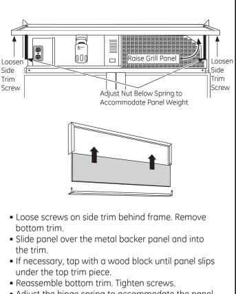
• Adjust the hinge spring to accommodate the panel weight, if necessary.
