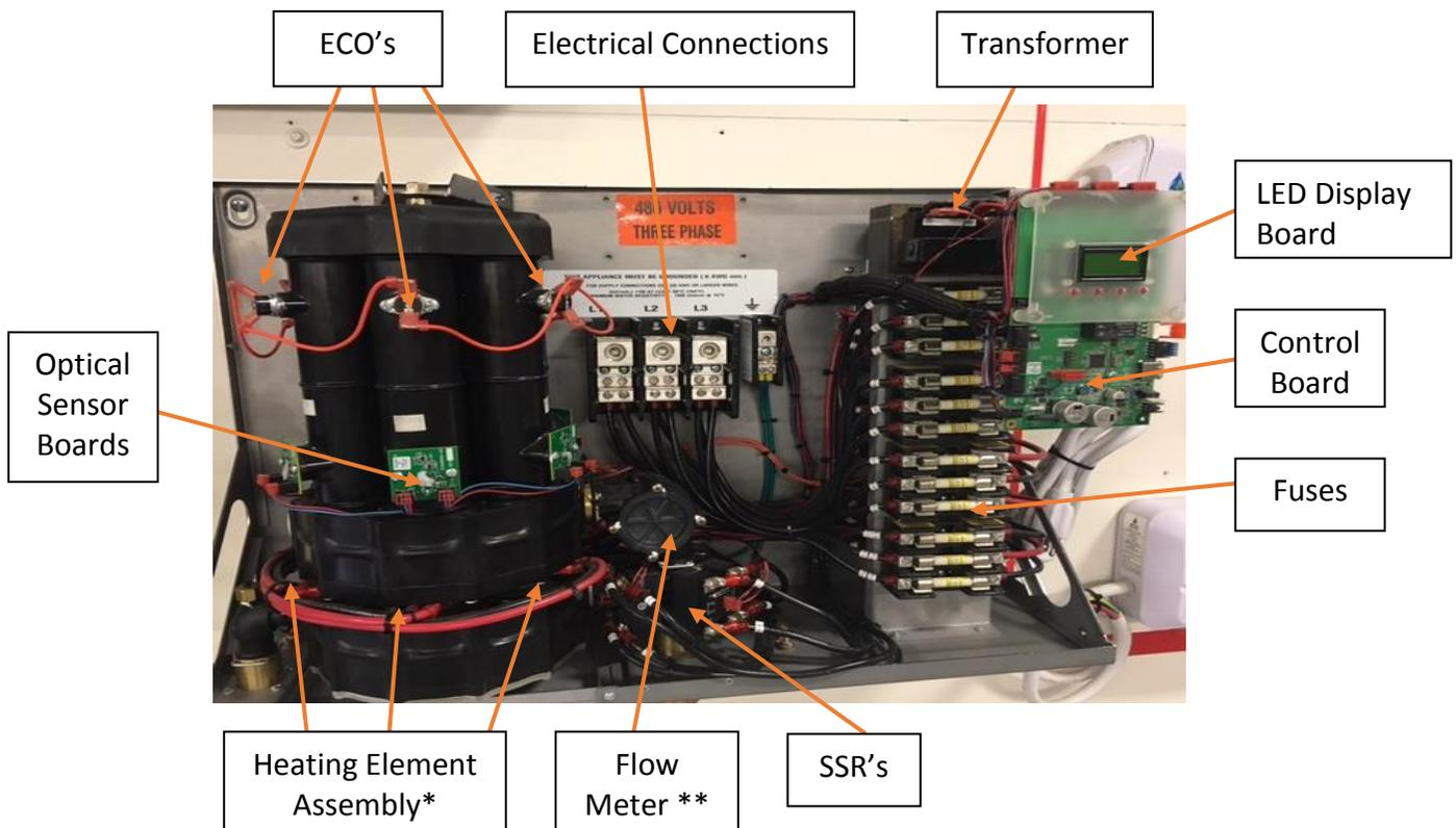
\* HEATING ELEMENT ASSEMBLY CONSISTS OF ONE HEATER CORE AND WIRE ELEMENT(S)
