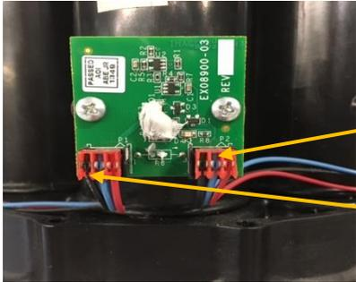
Lead placement: TEST BLUE AND BLACK SEPERATELY. PUT 1 LEAD ON BLUE WIRE ON P5 PLUG THEN OTHER LEAD GOES TO EACH BLUE WIRE ALONG OPTICAL SENSORS. REPEAT WITH BLACK WIRE.
