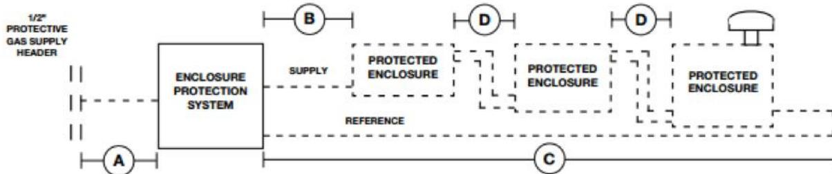
**\*NOTE:** TUBE AND PIPE SIZES ARE TRADE SIZES AND ARE NOT EQUAL IN INSIDE DIAMETERS. DO NOT SUBSTITUTE TUBE FOR PIPE WITH SAME TRADE SIZE.
