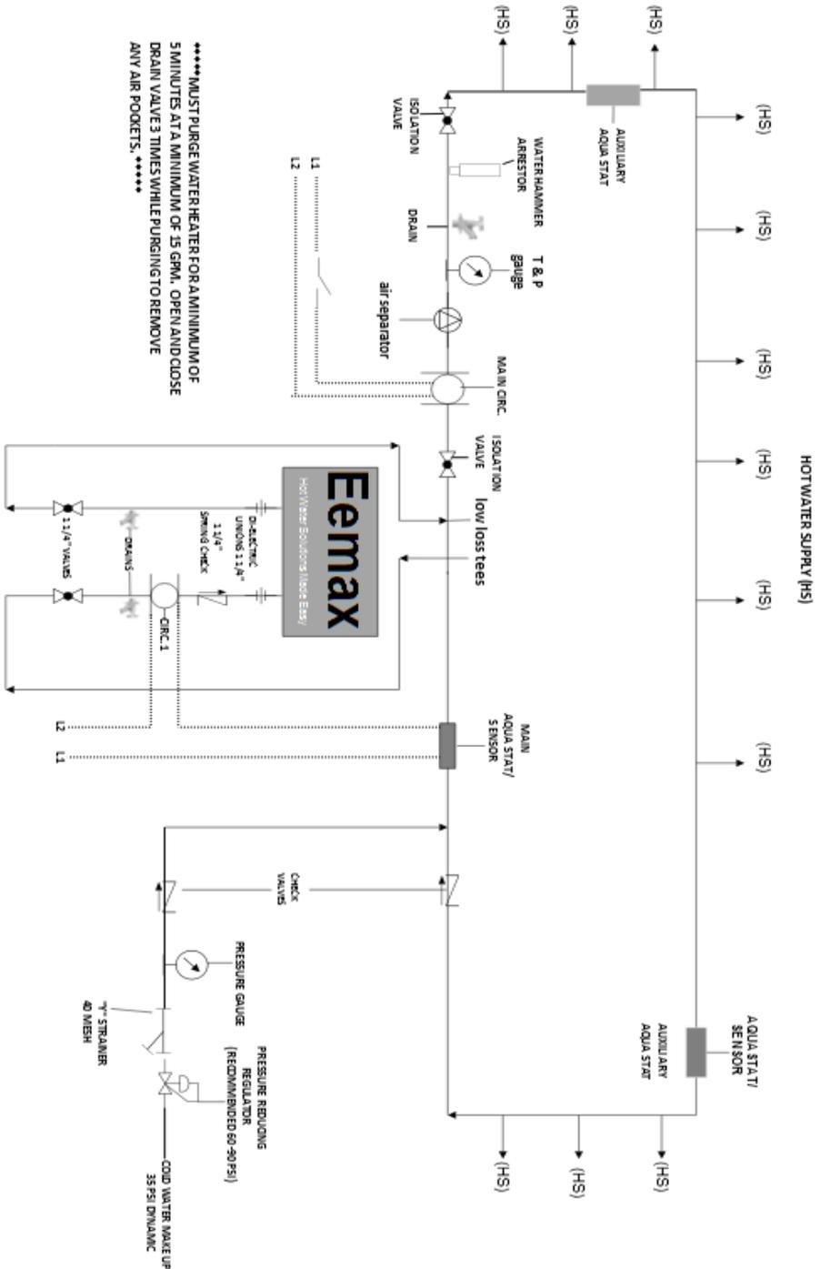
\*\*\*\*\*MUST PURGE WATERHEATER FOR A MINIMUM OF 5 MINUTES AT A MINIMUM OF 15 GPM. OPEN AND CLOSE DRAIN VALVE 3 TIMES WHILE PURGING TO REMOVE ANY AIR POCKETS.\*\*\*\*\*
