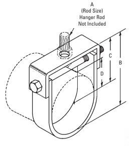
Bottom of pipe to top of hanger.
