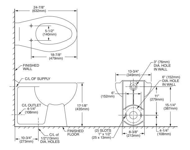
NOTES: \* VARIABLE — CHECK WITH MANUFACTURER OF FLUSHVALVE FOR PROPER ROUGH-IN DIMENSIONS. WASTE OUTLET SEAL RING MUST BE NEOPRENE OR GRAPHITE-FELT (WAX RING NOT RECOMMENDED). TO COMPLY WITH AREA CODE GOVERNING THE HEIGHT OF VACUUM BREAKER ON FLUSH VALVE, THE PLUMBER MUST VERIFY DIMENSIONS SHOWN FOR SUPPLY ROUGHING. FLUSH VALVE NOT INCLUDED AND MUST BE ORDERED SEPARATELY.
