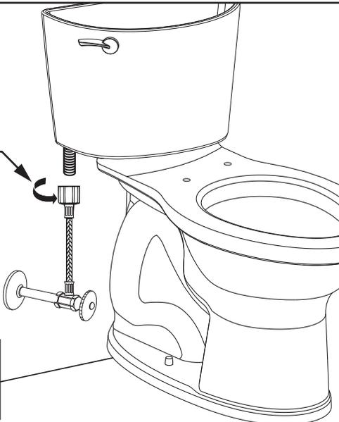
**!** **WARNING:** Overtightening of water supply line nuts could result in breakage and potential flooding. If the connection leaks after hand tightening, replace the supply line. Do not use any type of sealant on the water supply connection. Use of plumber's putty, pipe dope, or any other type of sealant will void the warranty.
