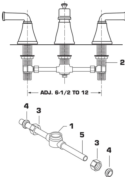
**NOTE** VALVE inlet is 3/4-inch NPT male connector.
