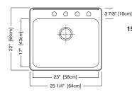
15SB.252284.073 Optional drilling: 4th hole on right
