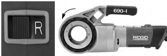
Figure 6B – R (REVERSE) (Counter-Clockwise) Switch Position
