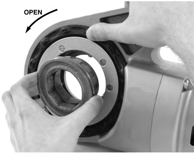
Figure 8 – Installing Adapter Into 690-I
