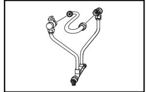
ANGLE BALL VALVE BY ANGLE CHECK VALVE (5/8" X 3/4" METER)
