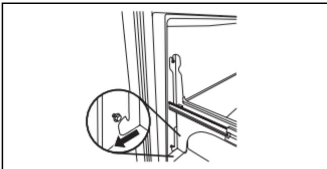
3. Completely tighten the four screws.
