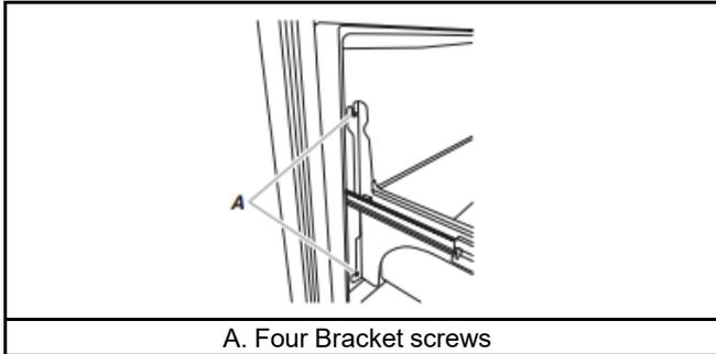
3. Lift drawer front upward and off the screws.
