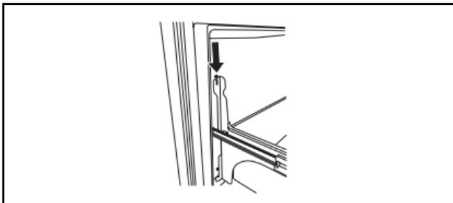
2. Pull the drawer brackets toward you to insert the two screws in the bottom of the drawer front into the brackets as shown below.
