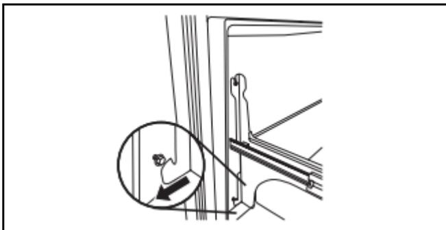
3. Completely tighten the four screws.
