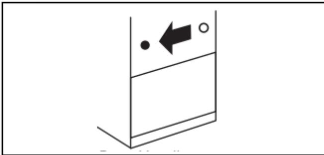
3. Remove the door stop. Move it to the opposite side of the refrigerator door as shown below.
