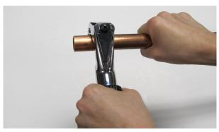
1. Make a clean cut onto the copper, CPVC, or PEX tubing. Deburr the edges to ensure that the outside diameter is free of sharp ridges.
