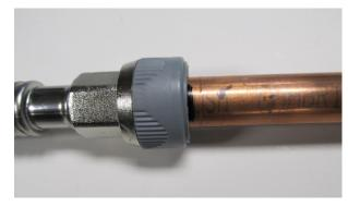
4. Insert the pipe into the fitting up to the 1.2" mark. Pull on the pipe to make sure that it is secure. Test the system for leakage before use.
