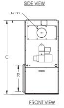
Note 1: Attach an external filter rack after cutting opening in side for return air duct connection. Either side can be used.
