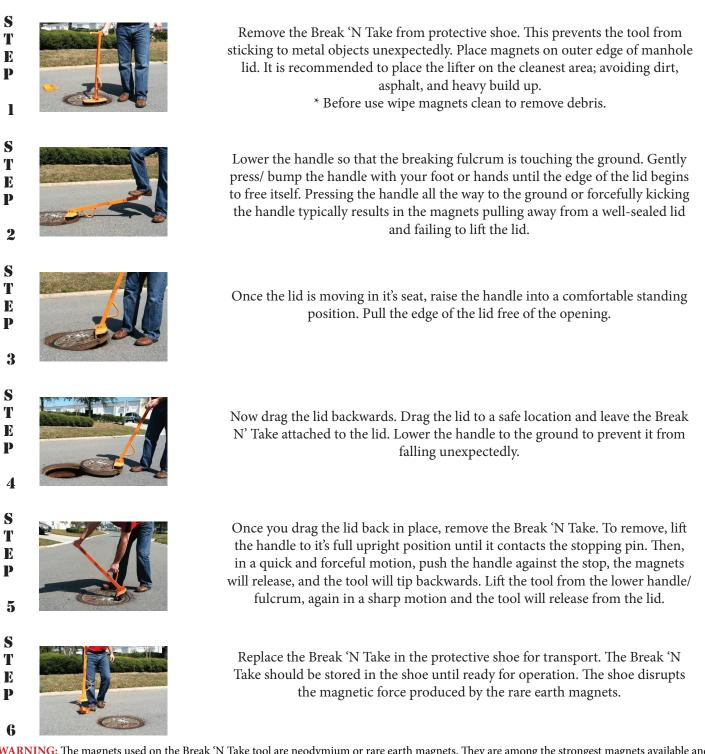
**WARNING:** The magnets used on the Break 'N Take tool are neodymium or rare earth magnets. They are among the strongest magnets available and exert enormous force. The energy in these magnets cannot be seen or felt by a person or on nonmetallic objects; however, caution should be taken around these tools. Use caution around credit cards, electronic devices, and metal objects.
