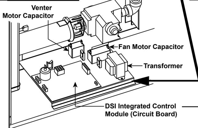
FIGURE 29. DSI Integrated Control Module (Circuit Board)
