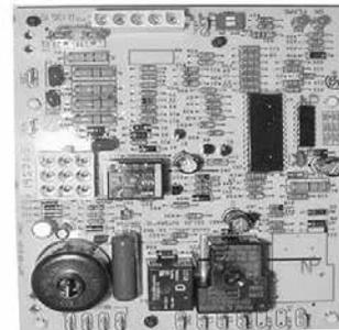
Only replaceable part is a type ATC or ATO 3-amp fuse (color code violet, PN 201685)
