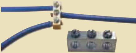
Copperhead's SnakeBite Pipe Burst Connector is a tin plated copper alloy made from 3/8" x 1/2" material with 1/4-20 slotted stainless steel set screws with oval points standard. We offer a three-hole connector for hooking up service and a two-hole connector for splice only. Wax tape is included with all pipe burst connector packages to eliminate moisture and prevent corrosion
