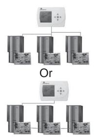
Two connections on DXM2 board to allow for multi-unit installation
