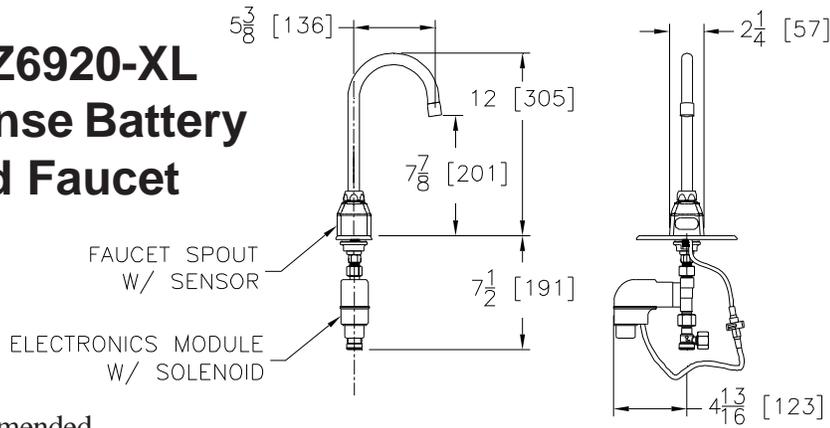
NOTE: Recommended through hole diameter to properly mount the spout/shank is 1-1/8" to 1-1/4".
