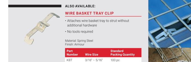
Use two clips per strut support for trays up to 12" (300mm). Use three clips per strut support for trays up to 18" (457mm) and add one clip per strut support for each additional 6" (150mm) of tray width.
