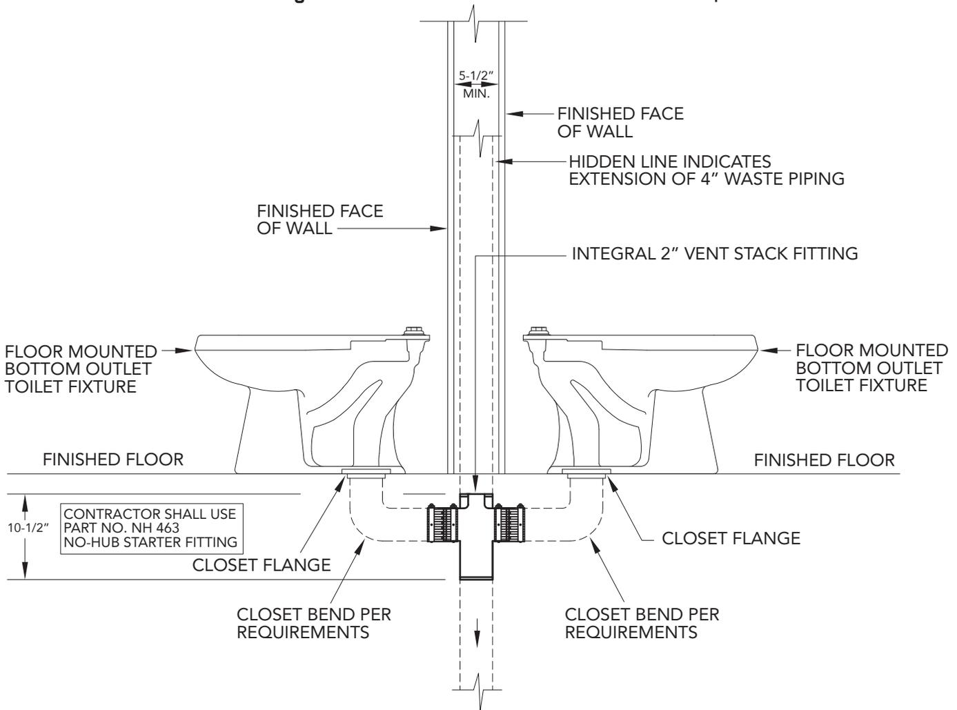
DOUBLE FITTING UNDER-SLAB - LEFT SIDE ELEVATION
