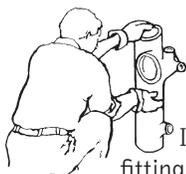
To determine if whether a closet fitting is a right hand or left hand configuration, stand the fitting up with the closet inlet facing you. If the opening is on your left, it is a **Left Hand** fitting. If the opening is on your right, it is a **Right Hand** fitting. Right Hand and Left Hand configurations do not apply for Double fittings.
