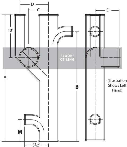
M & B dimensions must be measured from the bottom of the fitting.
