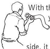
With the vented end toward you, hold the fitting so that you are looking into its length with the curved side up. If the vent is on your left side, it is a **Left** Hand fitting. If the vent is on your right side, it is a **Right** Hand fitting.
