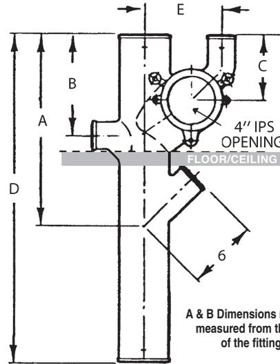
A & B Dimensions must be measured from the top of the fitting.
