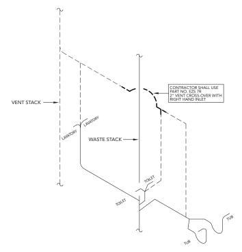
2" VENT CROSS-OVER FITTING RIGHT HAND RISER DIAGRAM
