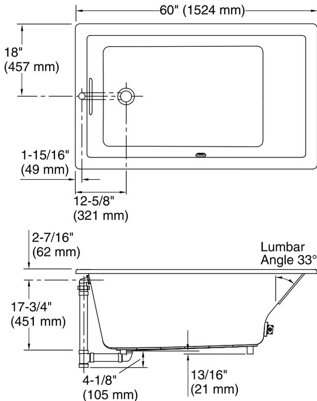
No change in measurement if connected with drain illustrated. (K-7272)
