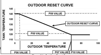
Figure 24 - Outdoor Reset Curve
