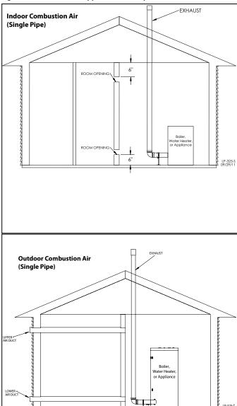
Figure 14 - Indoor and Outdoor Combustion Air - Single Pipe
