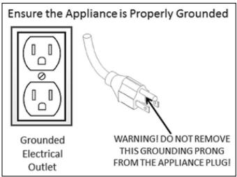
Figure 17 - Proper Grounding
