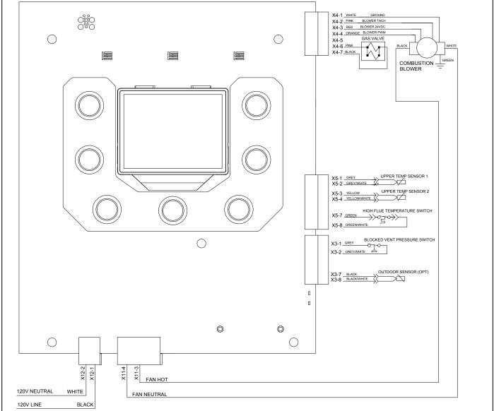
Figure 19 - Internal Wiring Diagram
