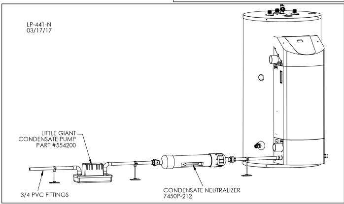
Figure 15 - Condensate Piping
