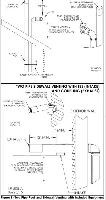
TWO PIPE ROOF VENTING WITH TEE (INTAKE)
