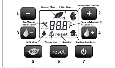
Figure 22 - Control Detail
