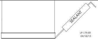
**Sealing Per NSF Standard 5 - For Sanitary Applications** Apply a 3/8" bead of RTV Silicone completely around the tank to seal the base to the floor and prevent seepage underneath.
