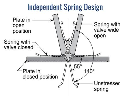
A spring design of the DUO-CHEK® (sizes 6" and larger) allows higher torque to be exerted against each plate with independent closing in response to the process stream. Testing has proved this action provides up
