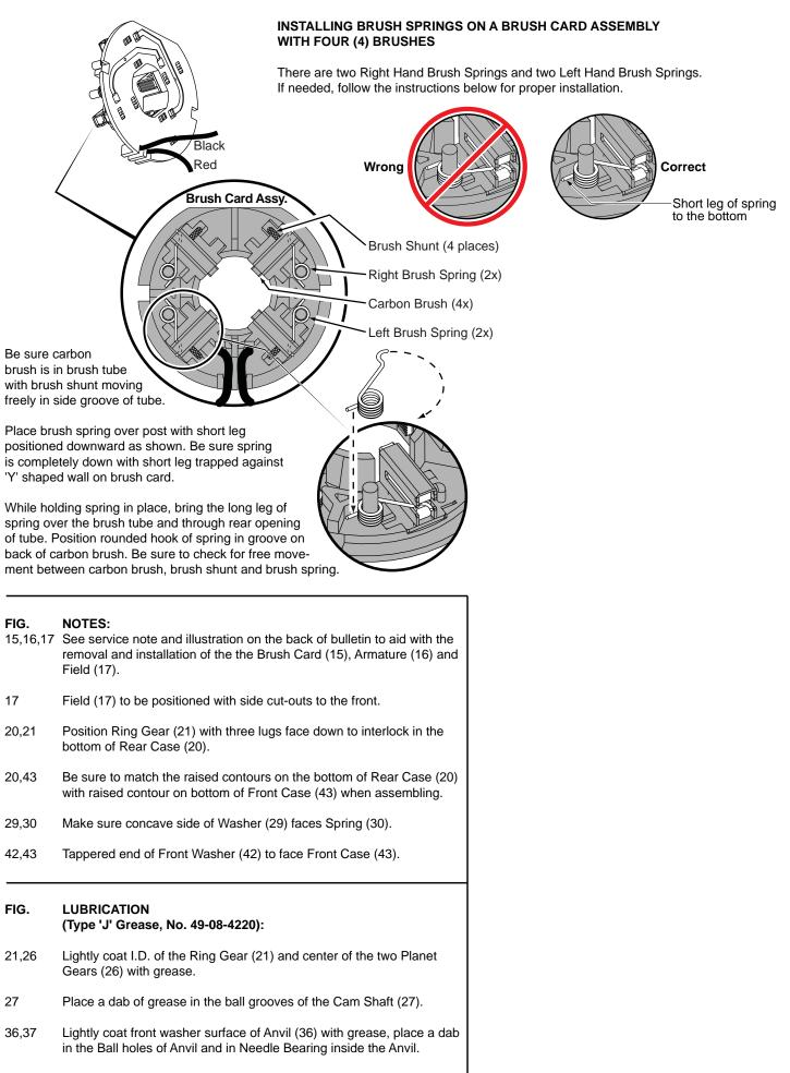
43 Coat inside grooves of Bushing (inside of 43) with grease.
