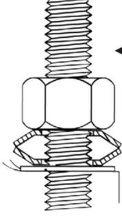
Smith-Blair® Belleville Washers (p/n 150115-000) must be used on PE pipe installations. Use of any other type of Spring Washer may cause product failure.
