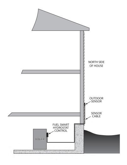
Before installation, determine the proper location for the sensor
