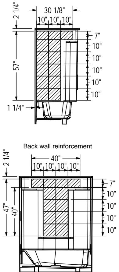
All dimensions are approximate. Structure measurements must be verified against the unit to ensure proper fit.
