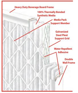
All Mark80-D and Hi-E 40 filters are designed with a consistent pleat shape on predetermined centers causing dirt to collect evenly over the entire surface of the media. Fully utilizing every square inch of media results in a slow, steady rise in resistance for maximum dust holding capacity.
