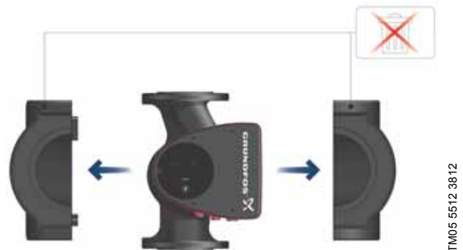
Fig. 3 Fitting insulating shells to the pump
