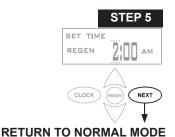
**STEP 5** – Next Regeneration Time (minutes): Set the minutes of day for regeneration using or buttons. Press NEXT to return to normal operation. Press (REGEN) to return to previous step.
