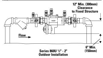
\*\*Metric Dimensions are nominal pipe diameter. This product is produced with NPT threaded end connections.
