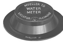
Cast iron meter pit covers - Inset pattern. 4" depth - recessed lid for installation in concrete or soil. **H-10811:** with MUELLER pentagon head. **H-10817:** with standard waterworks pentagon head. Touch read hole option available by adding -09. Double hole option available by adding -10.
