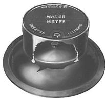
Cast iron meter pit covers - Double lid pattern for cold climates. 9-1/2" depth - non-recessed lid for parking installations. **H-10813:** with MUELLER pentagon head. **H-10818:** with standard waterworks pentagon head. Aluminum inner lid available by adding -00. Touch read hole option available by adding -09. Double hole option available by adding -10.
