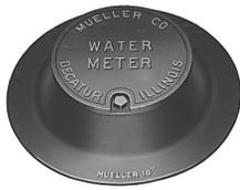
Cast iron meter pit covers - Regular pattern. 4" depth - non-recessed lid for parking installations. **H-10810:** with MUELLER pentagon head. **H-10816:** with standard waterworks pentagon head. Touch read hole option available by adding -09. Double hole option available by adding -10.
