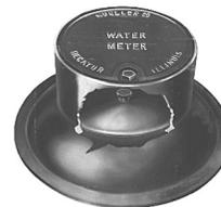
Cast iron meter pit covers - Double lid pattern for cold climates. 9-1/2" depth - recessed lid for installations in concrete or soil. **H-10812:** with MUELLER pentagon head. **H-10814:** with standard waterworks pentagon head. Aluminum inner lid available by adding -00. Touch read hole available by adding -09. Double hole available by adding -10.
